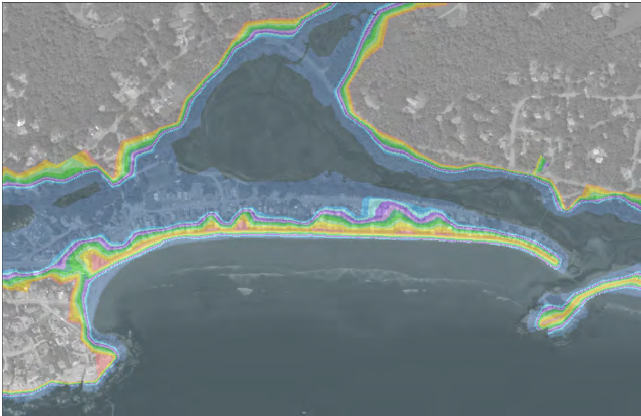
Flood Depths during a Coastal Flooding Event with a 1% Annual Coastal Flood Exceedance Probability (ACFEP) in 2070
