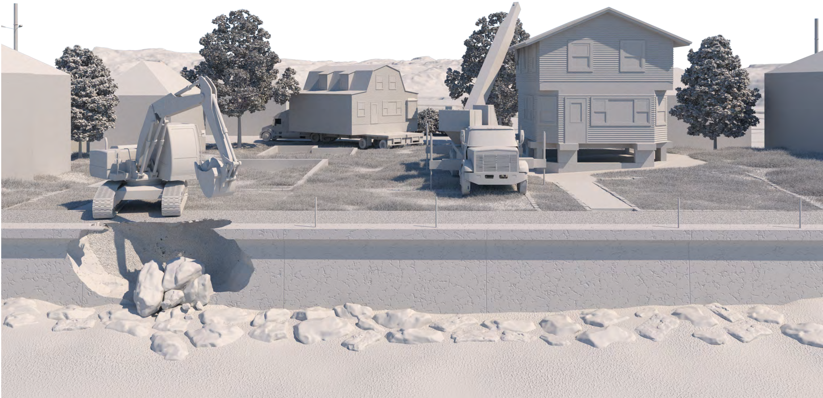
This rendering shows the process of relocating the cottages before deconstructing the seawall. APOCATOPIA, “Scenario 4: Relocate the Cottages,” 2024.
